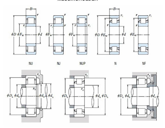
High quality cylindrical roller bearing with machined brass cage from the leading manufacturer TIMKEN. Featuring the TIMKEN EMA design. A premium land-riding cage, unique internal geometries, enhanced surface finishes and a compact design. All this adds up to longer life, improved uptime and reduced maintenance costs.
